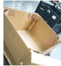
Sleeve designed with removable wood support
